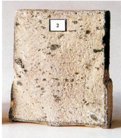
[Above: a concrete block that was coated with KF-B (at left) and another concrete block without the KF-B coating (at right). Both blocks were submerged in a 25% Sulfuric Acid solution - a highly corrosive acid that is present in sewer systems. The unprotected block shows significant corrosion and mass loss]
