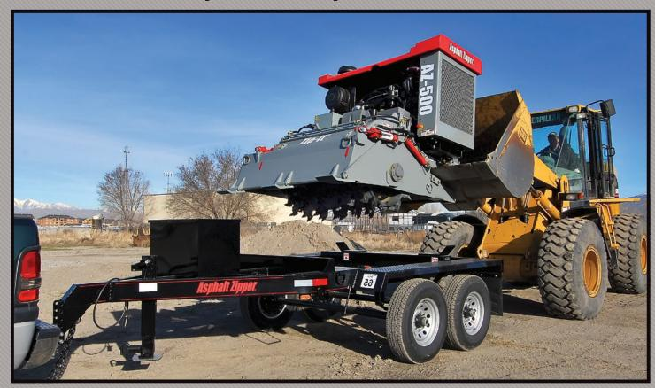
Asphalt Zipper's patented Versa-Mount™ universal bucket mounting system allows the Zipper to fit the widest possible range of loaders, backhoes, and skid steers. The Asphalt Zipper® mounts securely in just minutes. Optional quick-connect system also available.
