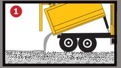
Spread additional material or additive (crushed rock, cement, fly ash, lime, etc.).
